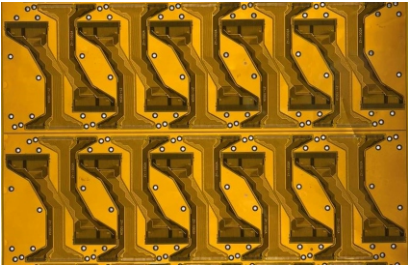
外形切割 Shape cutting
